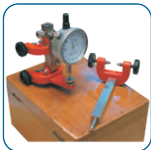
Mechanical Extensometer Least Count 0.01 mm
